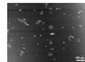
Figure 8. AFM image of DNA-C at pH 5.0 liquid (Z 5 nm).
